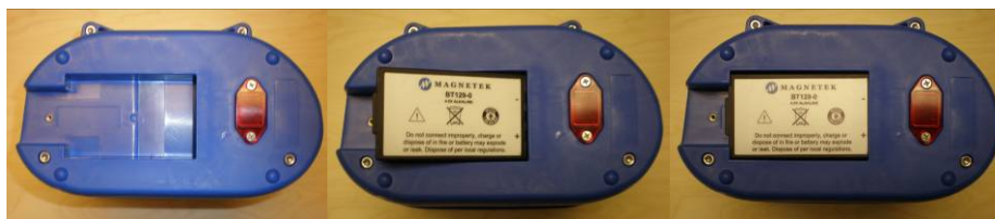
Figure 4: Installation of Battery Pack into MLTX2 transmitter
